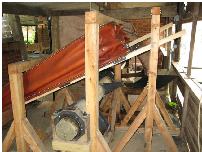
The bellows operated from below by cams
