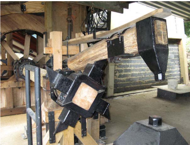
The half scale belly helve hammer
